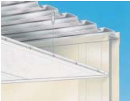
Cutaway section of corrugated roof deck and acoustical ceiling.
