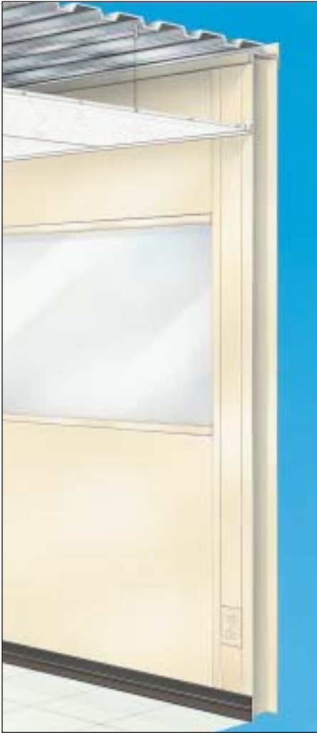
Ceiling suspended from roof deck.
