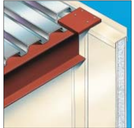
Loadbearing roof beam.
